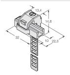
Mounting bracket for mounting magnetic field sensors on round cylinders; cylinder diameter: 63...130 mm; material: PA 6I/6T / nickel silver; fire-hazard classification acc. to UL94 - V2
