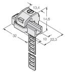
Mounting bracket for mounting magnetic field sensors on round cylinders; cylinder diameter: 130... 250 mm; material: PA 6I/6T / nickel silver; fire-hazard classification acc. to UL94 - V2
