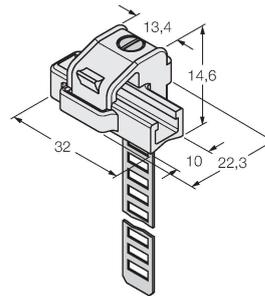
Mounting bracket for mounting magnetic field sensors on round cylinders; cylinder diameter: 25...63 mm; material: PA 6I/6T / nickel silver; fire-hazard classification acc. to UL94 - V2
