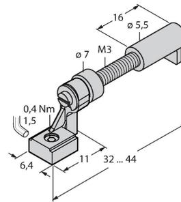
Accessories for fine-tuning of the switching point on T-groove cylinders; snap-lock mounting in the BIM-UNT sensor fixture; suited for multiple use; material: Metal/plastic
