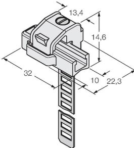
Mounting bracket for mounting magnetic field sensors on round cylinders; cylinder diameter: 63...130 mm; material: PA 6I/6T / nickel silver; fire-hazard classification acc. to UL94 - V2
