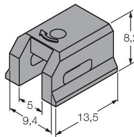
Mounting bracket for mounting magnetic field sensors on dovetail groove cylinders; groove width: 9.4 mm; material: PPS
