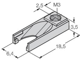
Accessories for finetuning the switchpoint on T-groove cylinders; snap-locked in the BIM-UNT fixture; suited for multiple use; material: plastic
