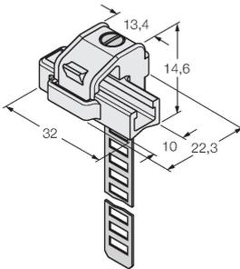
Mounting bracket for mounting magnetic field sensors on round cylinders; cylinder diameter: 8...25 mm; material: PA 6I/6T / nickel silver; fire-hazard classification acc. to UL94 - V2
