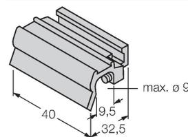
Accessories for mounting the sensors BIM-INT and BIM-UNT on tie-rod cylinders; Cylinder diameter: 50...63 mm; material: Aluminium; Further mounting accessories for other cylinder diameters on request
