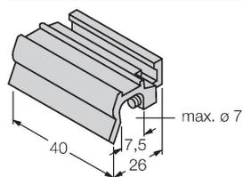
Accessories for mounting the sensors BIM-INT and BIM-UNT on tie-rod cylinders; Cylinder diameter: 32...40 mm; material: Aluminium; Further mounting accessories for other cylinder diameters on request
