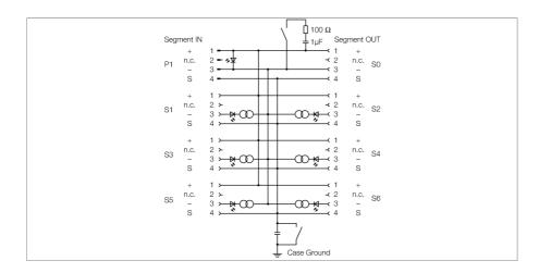
The 6-channel junction box JBBS-48SC-M613/3G is designed for PROFIBUS-PA systems.
