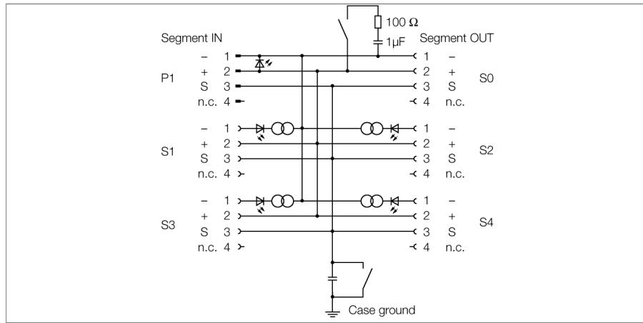
The 4-channel Ex junction box JBBS-49SC-M413/EX is designed for FOUNDATION™ fieldbus systems.
