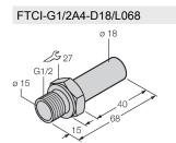
6870150 Adapter for G1/2 thread made of stainless steel A4 (1.4571/AISI 316Ti)
