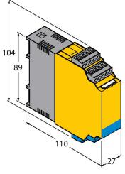
Ex signal processor for Ex flow sensors from the FC...-NAEX... product series; operating voltage 20...250 VAC; LED bar for displaying flow speed and medium temperature; IO-Link device with relay outputs for flow, temperature and errors
