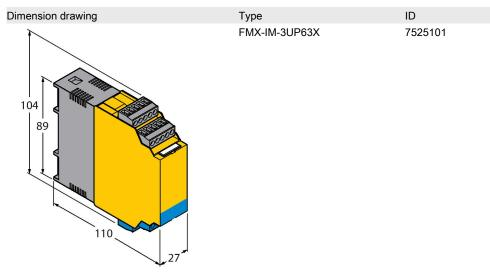
Ex signal processor for Ex flow sensors from the FC...-NAEX... product series; operating voltage 20...30 VDC; LED bar for displaying flow speed and medium temperature; IO-Link device with transistor outputs for flow, temperature and errors
