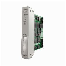
The analog input module Al43Ex is used for the connection of potentiometers in 3 or 4-wire technology. If 3-wire potentiometers are used, the terminals at the module rack have to be bridged. Resistance measurements, i.e. the evaluation of potentiometers with a 2-wire connection, is not possible.
