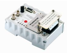
The optocoupler OC11Ex/2G.2 converts the PROFIBUS-DP signals on copper cables into optical signals. The bus signals can therefore be transmitted from the safe area to the Ex area over long distances without potential or interference. When using fiber-optic cables, the maximum baud range is 2500 m for OM1 (62.5/125-µm) cables and 1500 m for OM2 (50/125-µm) cables.
