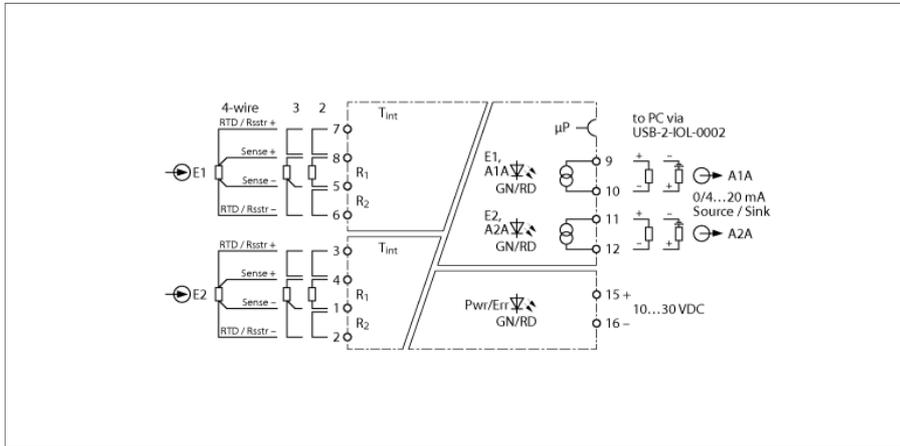
The temperature transducer IM12-TI01-2RTDR-2I-C0/24VDC transmits temperature-dependent measured values galvanically isolated. The devices are suitable for operation in zone 2.
