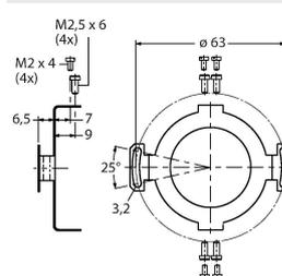
Stainless steel flex mount coupling for hollow shaft encoders, reference diameter 63 mm, for applications with high demands on accuracy
