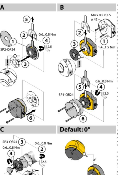
Extensive range of mounting accessories for easy adaptation to many different shaft diameters. Based on the functional principle of RLC coupling, the encoder is immune to magnetized metal splinters and other interferences
