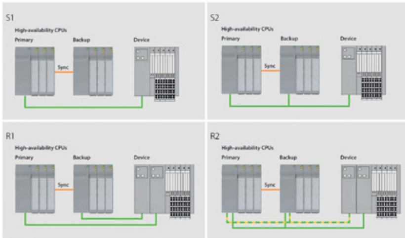
Redundancy principles: S1 is a simple connection, i.e. no redundancy; if a Profinet device communicates with the primary controller and its backup via this connection, this is classified as S2 – very high and maximum availability is offered only with R1 and R2 system redundancy, which also require dual systems on the field side
