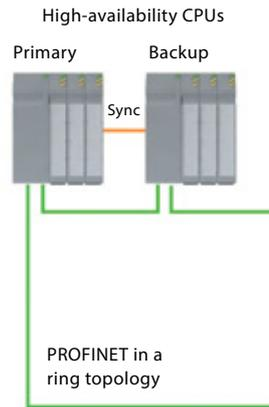
are normally provided with redundancy in order to ensure safe plant operation. If one device or connection fails, the otherwise inactive backup solution is activated. Planners implement these complex or limited redundant systems in accordance with the relevant requirements – both on the physical device level as well as in the underlying programming logic.
