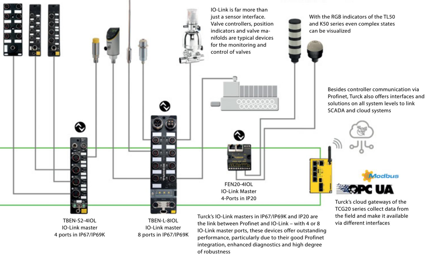
IO-Link is far more than just a sensor interface. Valve controllers, position indicators and valve manifolds are typical devices for the monitoring and control of valves
