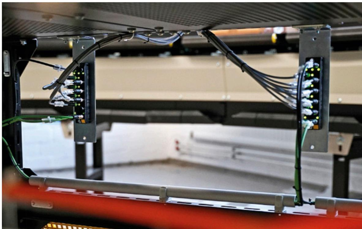
To ensure efficient operation in spite of the large number of sensor and actuator signals in intralogistics systems, Turck has developed a block module with universal channels that can be used as inputs or outputs as required
