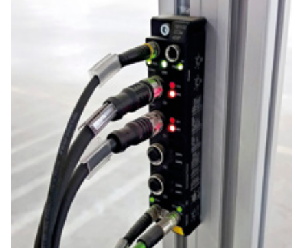
Turck's TBEN-S multiprotocol I/O modules ensure reliable communication between the PTL110 and the WMS
