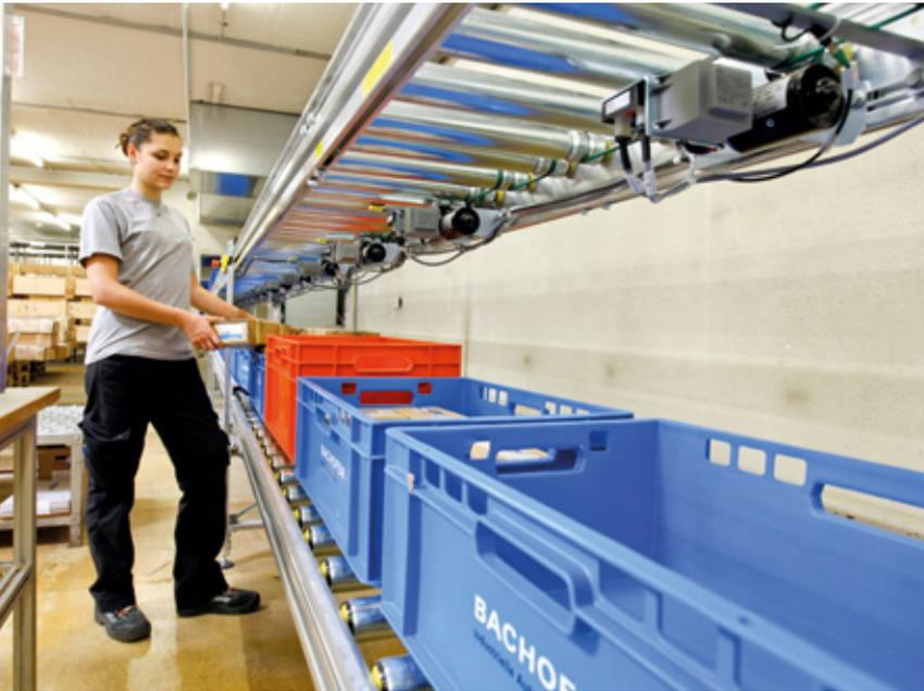
In applications using many read/write heads, wiring effort is reduced by the possible cascading of the RFID interfaces
