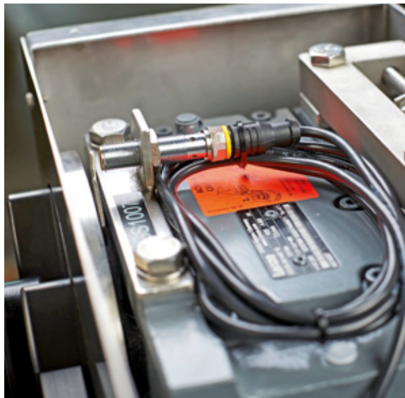
The BI6U-M12-IOL6X2 IO-Link sensor detects the correct position of the rotation unit via the switch lug
